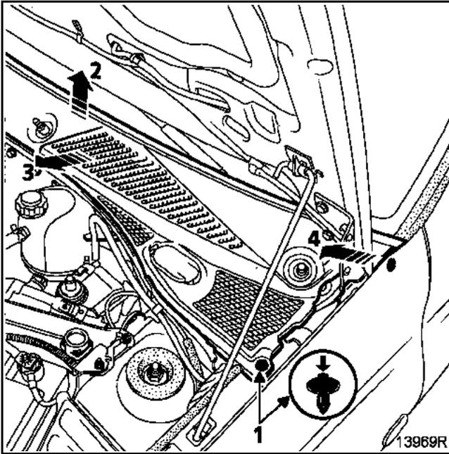
Press the shaft in the centre of the rivet (1) and lower it by **5 mm** maximum, using a **T10** or **T20** torx screwdriver.
