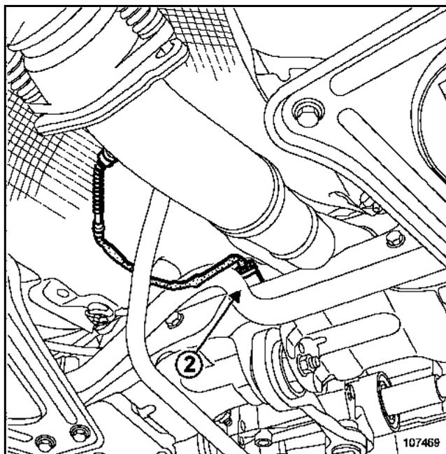
Disconnect the upstream oxygen sensor connector (2)
