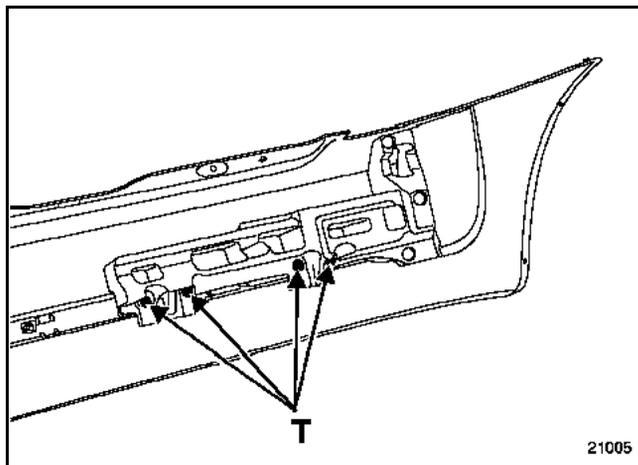
Remove the clips (T), then remove the impact absorber.
