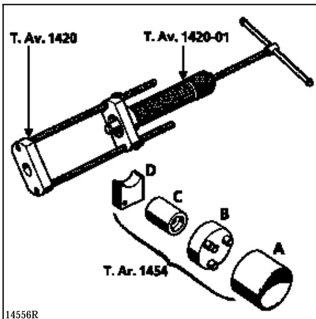
Fit the required tooling in place, which is the rings (A), (C) and the spacer (D) from tool **T. Ar. 1454** as well as tool **T. Av. 1420** and **1420-01** onto the rubber bush to be removed .
