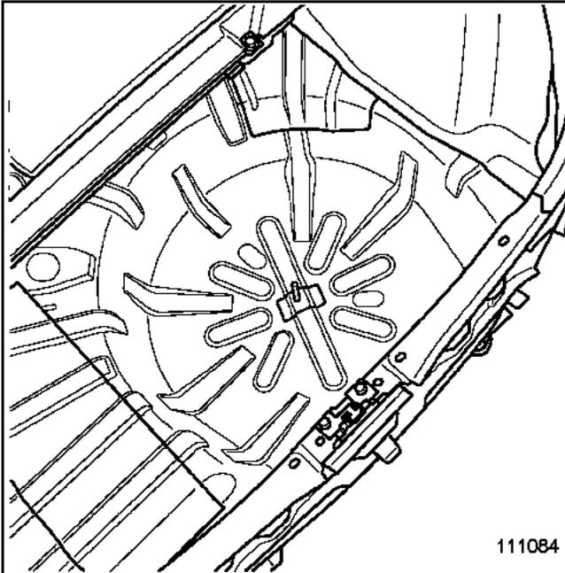
Cut the floor which lies over the spare wheel compartment.
