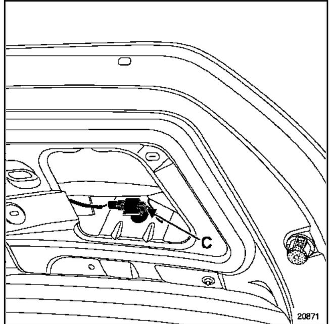
Disconnect the male connector (C), then remove the female connector from the clip.
