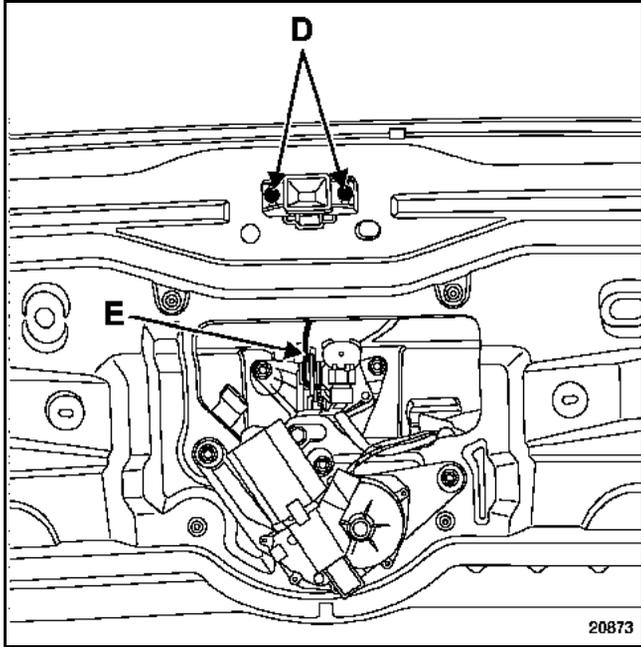
Remove the two bolts from the lock (D).
