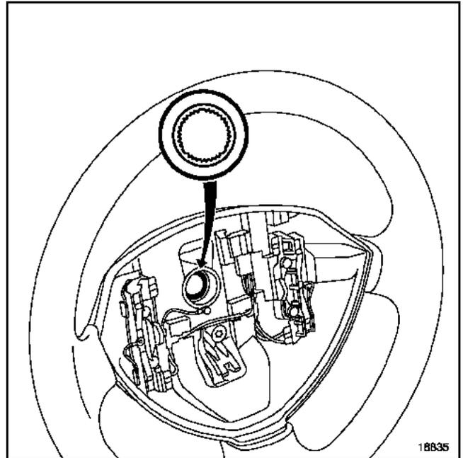
**IMPORTANT:** the steering wheel splines are made so that the wheel can be fitted in one position only. The steering wheel should slip freely into the splines.
