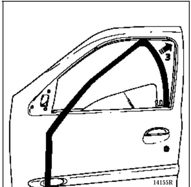
Insert the rear vertical section of the guide into the door box section.
