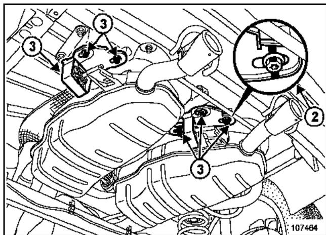
Mark the position of bolts (2) on the brackets.
