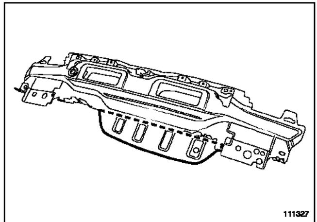
Cut the rear end panel by the spare wheel compartment, under the bumper mountings.
