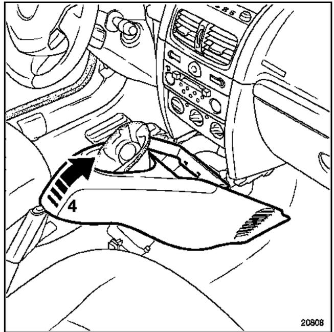
Remove the console from the gear lever position (4).
