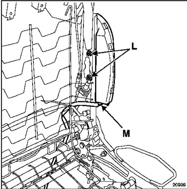
Tighten the two air bag nuts (L) to a torque of **(8 Nm)**.
