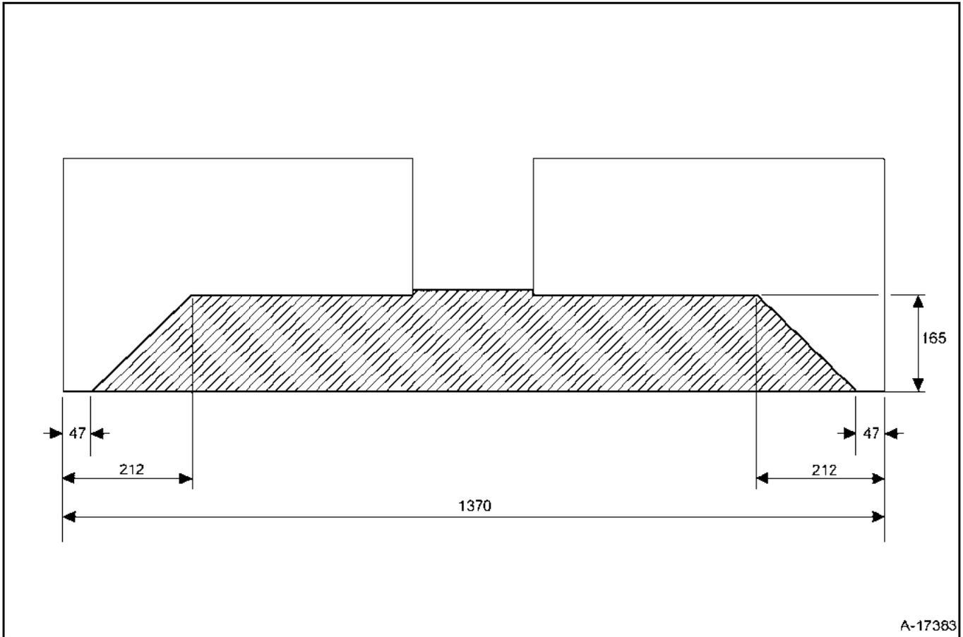
The rear floor insulation is supplied in one piece and must be cut in two. The margin for the cutting line is  $\pm 3.0$  mm.
