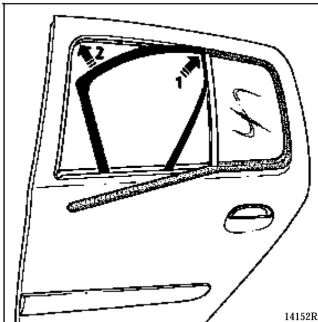
Insert the two vertical sections in the door box section.
