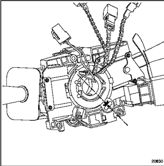
Check that the rotary switch is correctly positioned by making sure that the mark "O" is located right on the steering shaft.
