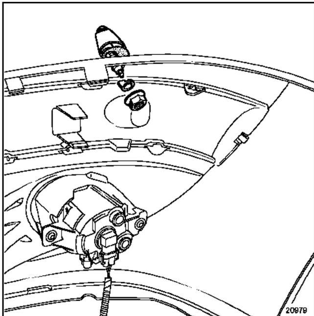
Fit the jet with its shim and seal.
