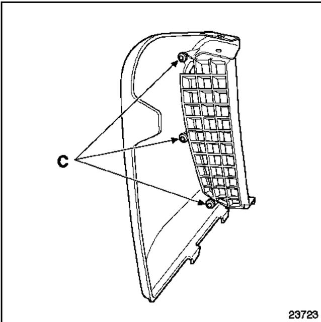
Remove screws (C) and release the grille.
