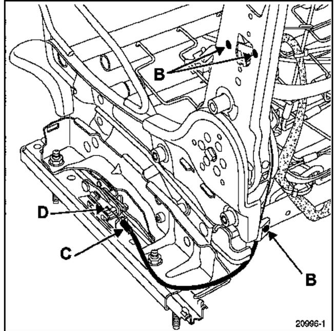
Drill out the three rivets (B).
