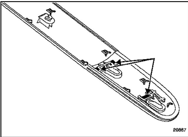
Remove the three clips, and then remove the badge using a small screwdriver.
