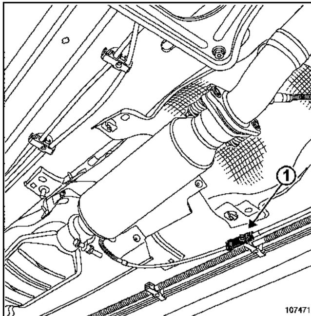
Disconnect downstream oxygen sensor connector (1).
