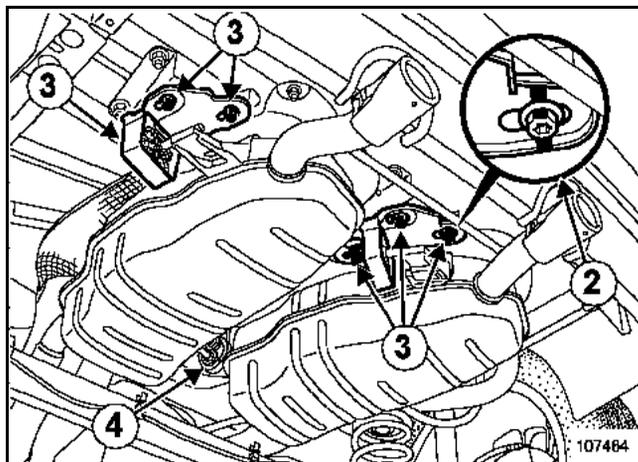
Check that there is **15 mm** clearance between the grooves and the edges of the silencers made in the rear bumper.
