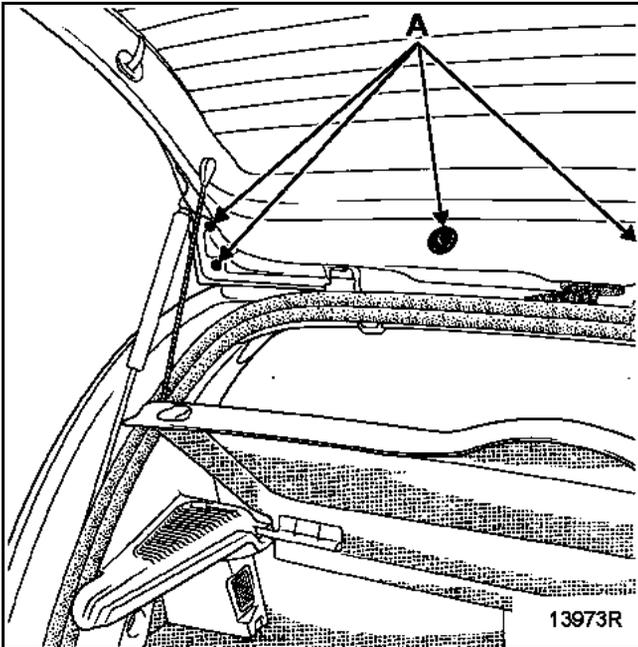
Remove mounting bolts (A) from the tailgate spoiler.
