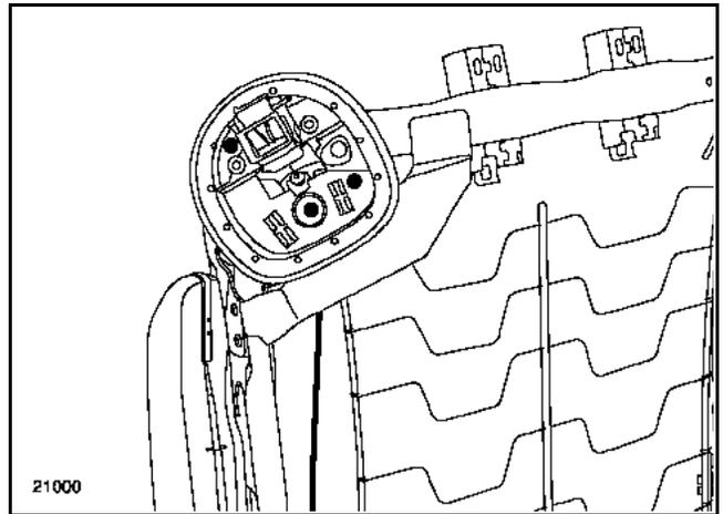
Drill out the three rivets, then remove the opening control.
