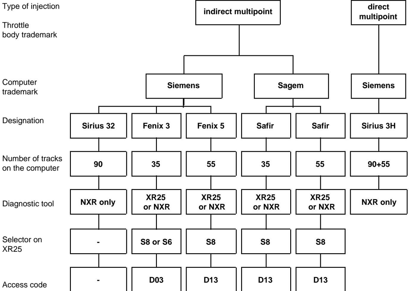
Function #90 enables you to find out the diagnostic to be used after communicating again (D03 or D13) with the computer.
