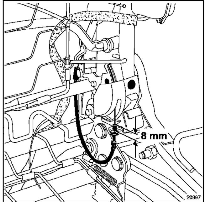
The setting of the two stop washers must be respected **(8 mm)** when refitting the seatback unlocking cable.
