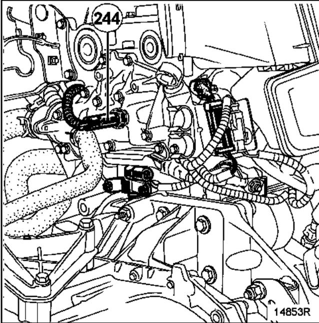
**244** Coolant temperature sensor (injection and coolant temperature displayed on the instrument panel).
