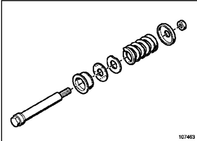
Observe the direction of fitting of the catalytic converter upstream mounting washers.
