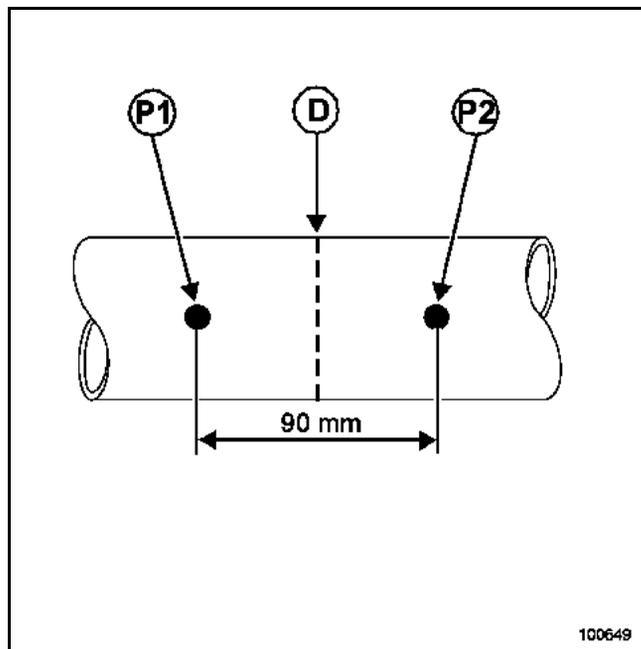
Before cutting the pipe, mark the area (D) between marks (P1) and (P2).
