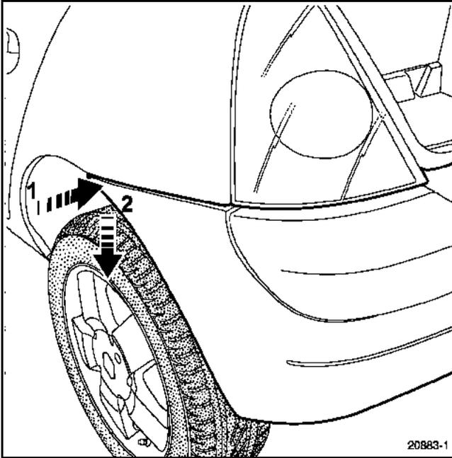
Remove the corner of the bumper (1), then tilt the bumper (2).
