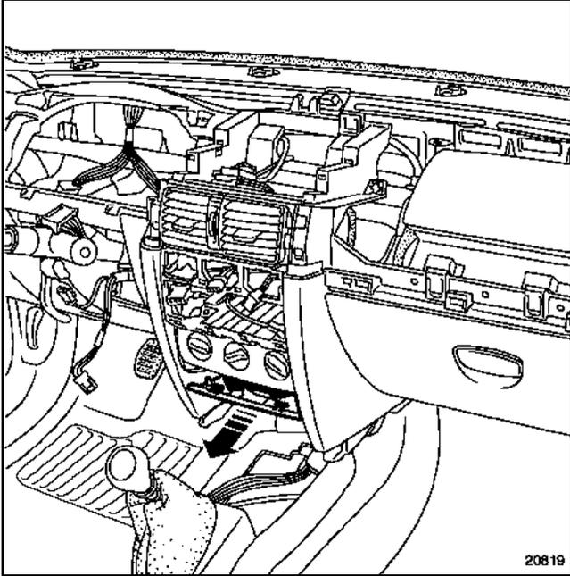
Release the Carminat speaker support and disconnect the connector.
