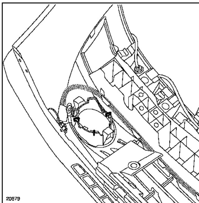
Remove the three clips then remove the fog light mounting.
