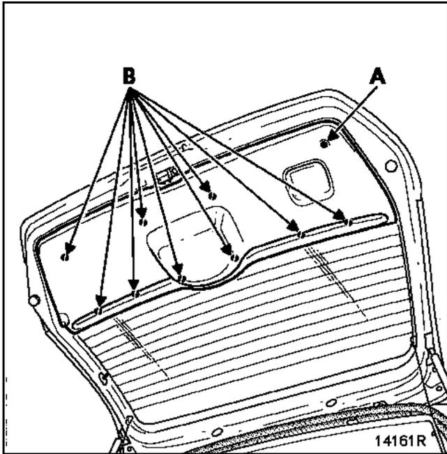
Remove fixing screw (A).
