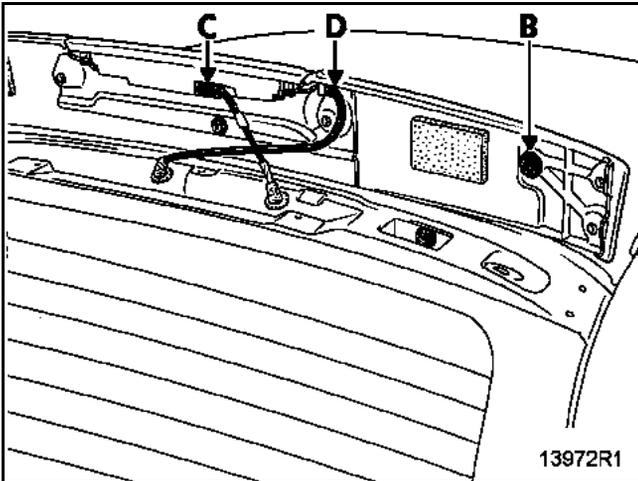
Unclip spoiler (B) by pulling it upwards.
