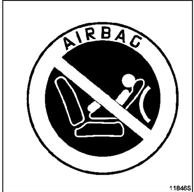
If you need to remove a dashboard fitted with a passenger air bag, you must replace the sticker shown above after refitting (on the side of the dashboard). This label comes in the **Parts Stores** set, part no. **77 01 205 442**.
