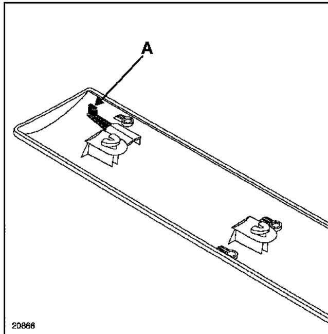
Before refitting the mountings, it is necessary to pull out the tab (A) slightly to ensure that the mounting is locked.
