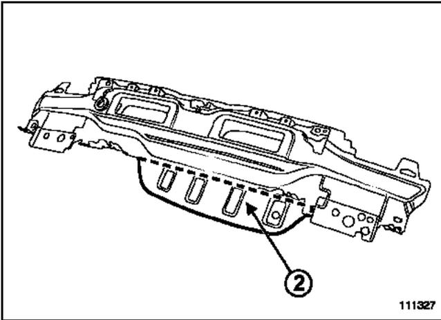
Cut the lower section of the rear end panel (2) by the spare wheel compartment, under the bumper mountings.
