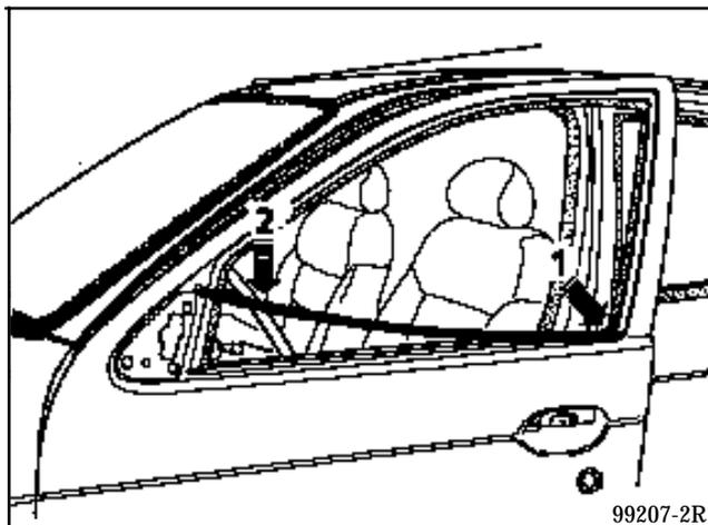
Fit the weatherstrip at the rear of the front door and push it towards the rear (1).
