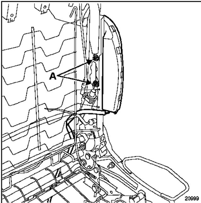
Remove the two fastenings (A), then partially release the air bag.
