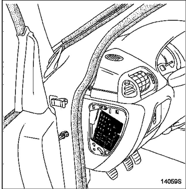
Use a **20 A** fuse, available with the replacement fuses, and reconnect it in position **no. 29** before delivering the vehicle to the customer.
