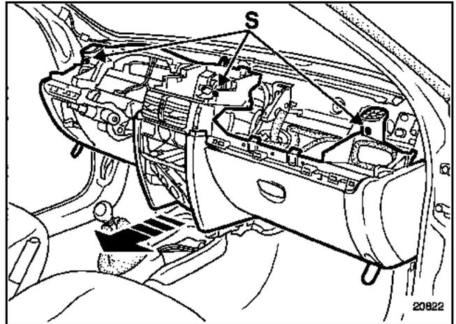
Remove the three upper dashboard mounting bolts (S).
