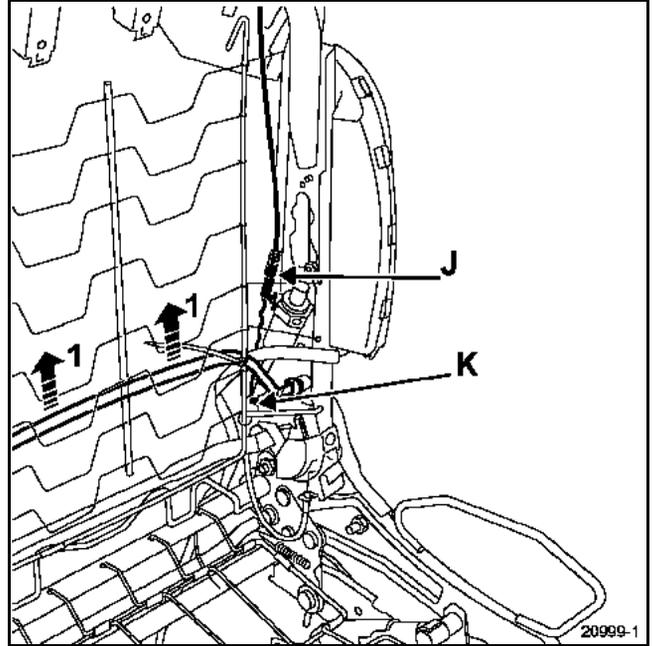
Press (1), then release the stop clip (J) and the cable (K).
