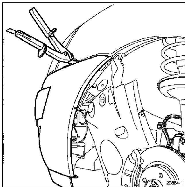
**IMPORTANT:** before removing the side part of the bumper, protect the front wing and the bumper with masking tape.
