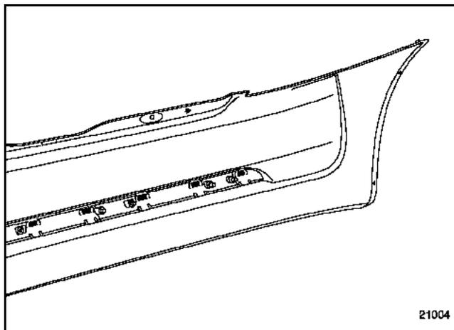
Remove the clips, then remove the strip.
