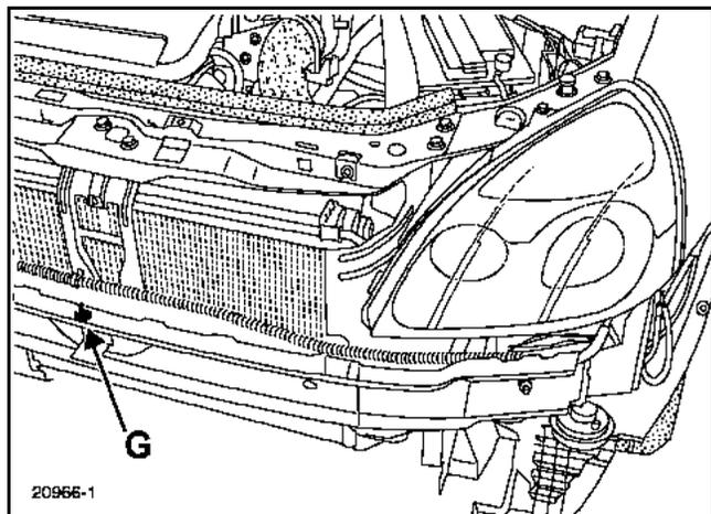
Before offering up the bumper, check the indexing guide (G), which ensures that the bumper is in the correct position.
