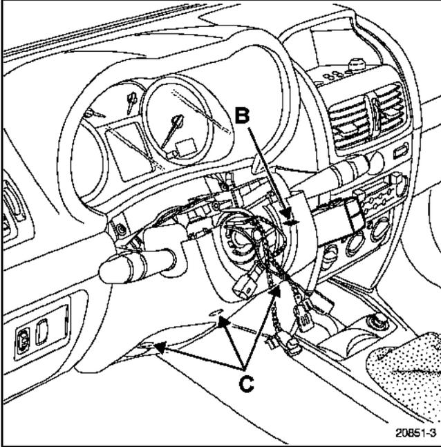
Press on clip (B) with a flat screwdriver, to release the radio satellite control.
