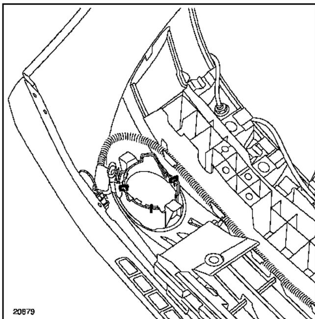
Clip the fog light mounting to the bumper (pig's snout light clip) using the clip-fitting pliers (**Car. 1521**).
