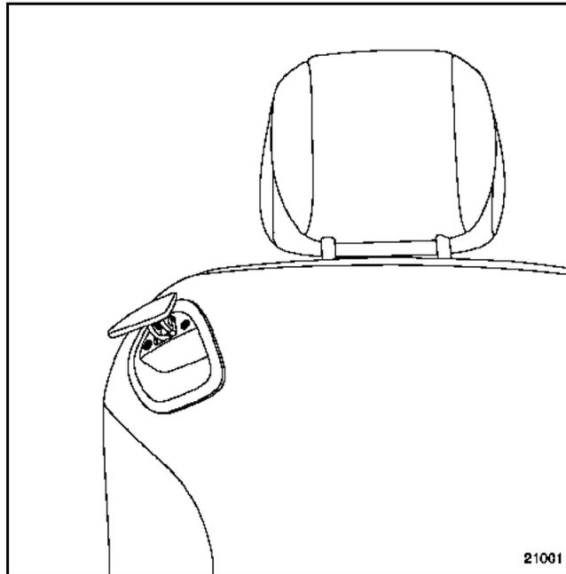
Remove the two mounting bolts from the unlocking control.
