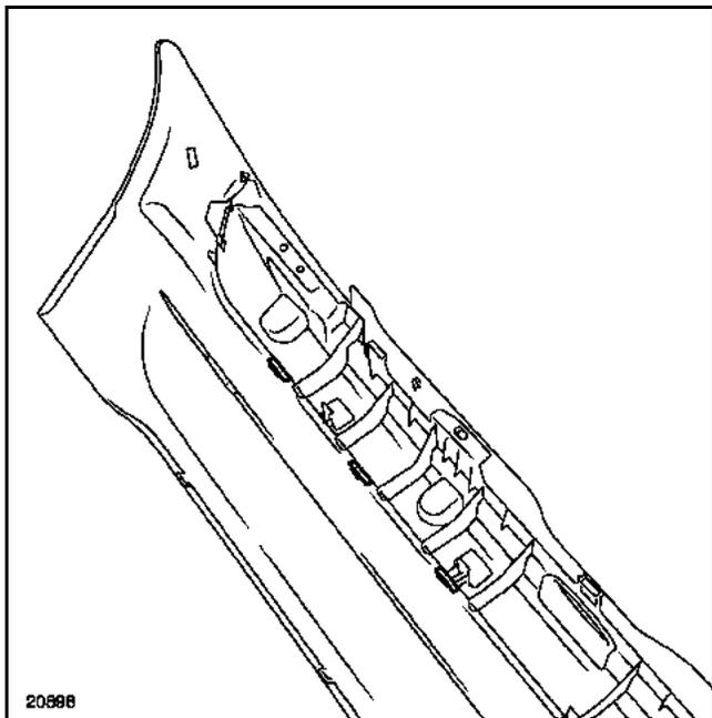
Unclip the strip mountings, then remove the strip.
