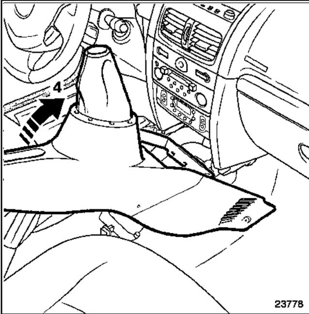
Release the console (4) at the gear lever and handbrake gaiters.
