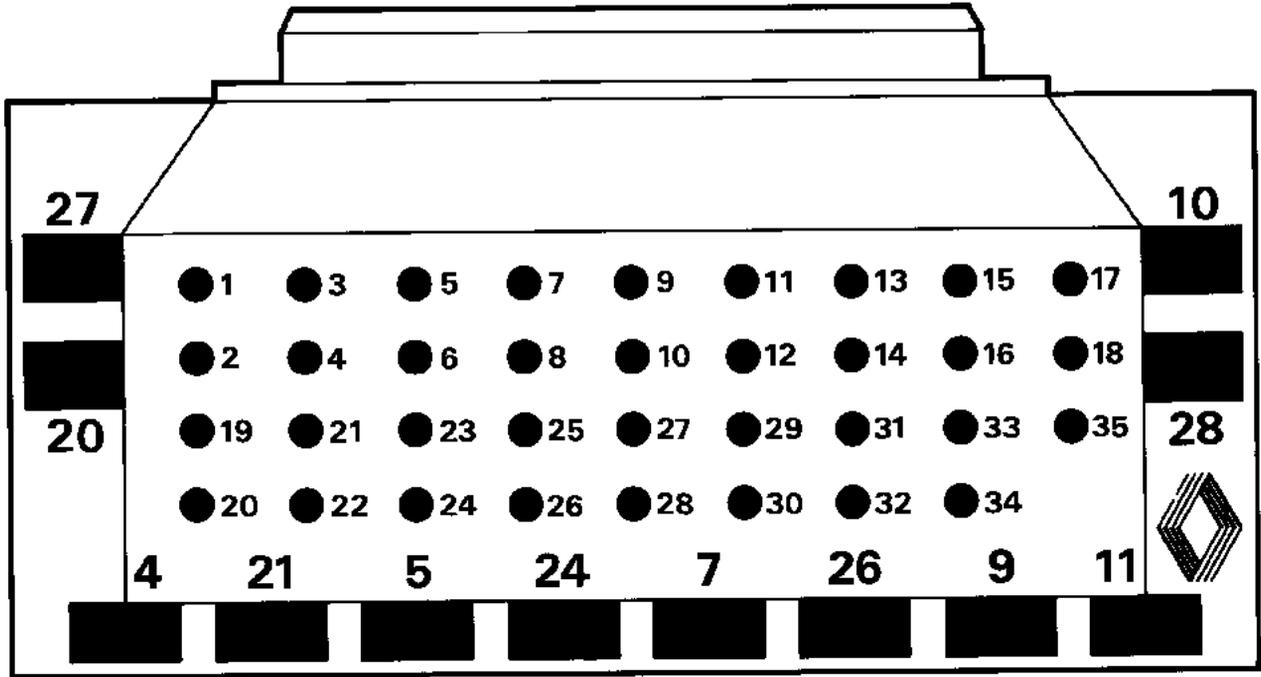
Bornier **MS 1048** is a 35 track base with a printed circuit on which there are 35 copper-coated areas, numbered from 1 to 35.
