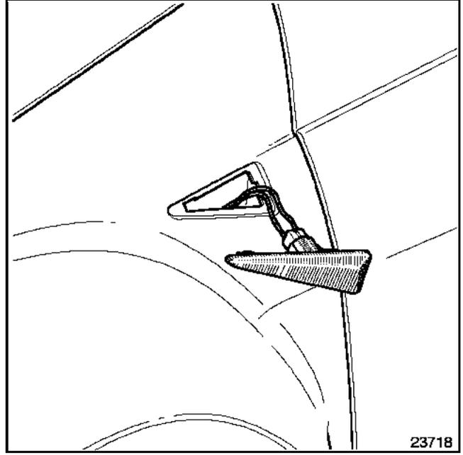
Unclip the side mounted indicator repeater.
