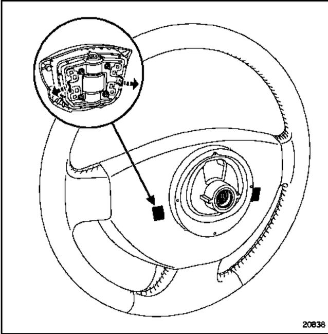
Unclip the air bag from the steering wheel using a flat screwdriver.
