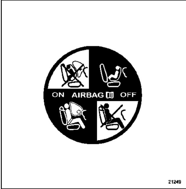
If you need to replace a dashboard fitted with a passenger air bag, you must replace the sticker shown above after refitting (on the side of the dashboard).
