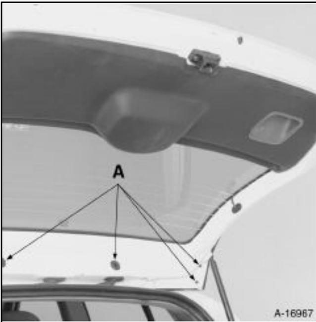
Remove the mounting bolts (A) from the spoiler on the tailgate.
