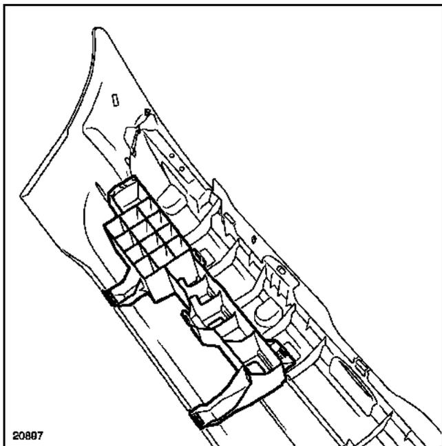
Unclip the four mountings and remove the impact absorber using a flat screwdriver.
