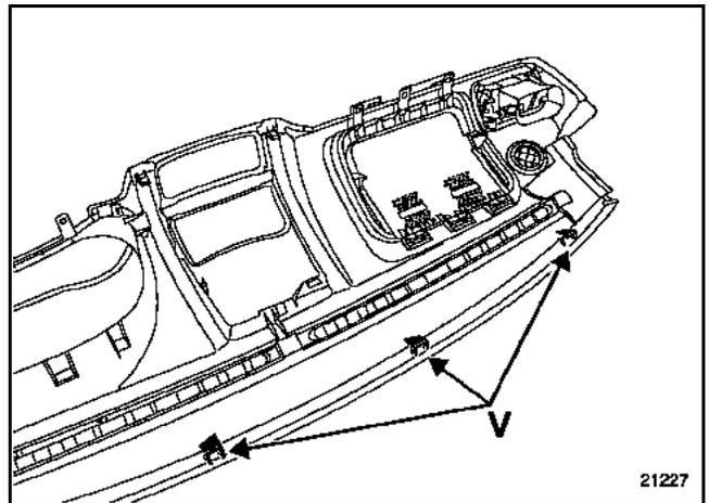
**IMPORTANT:** it is crucial to check that the retaining clips (U) and (V) are in good condition before replacing the cover.
