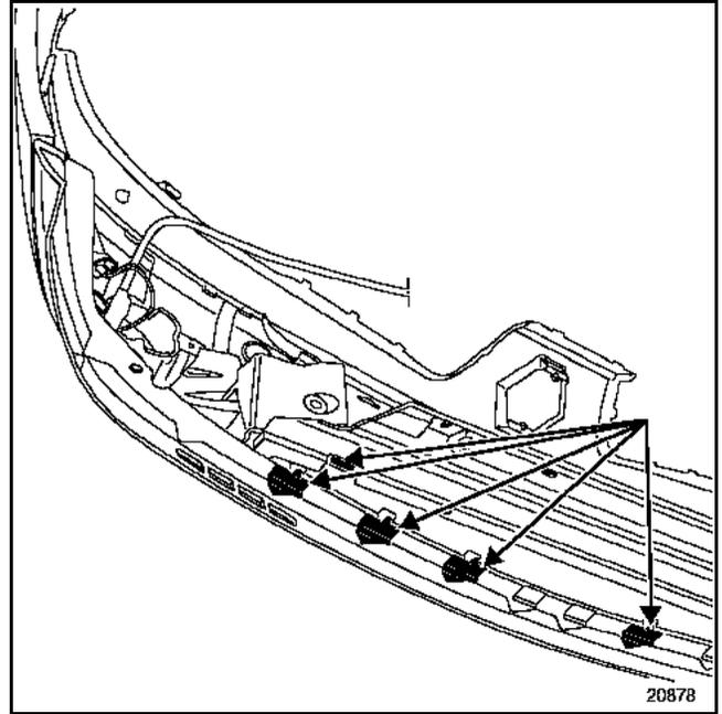
Remove the clips, then remove the housing.
