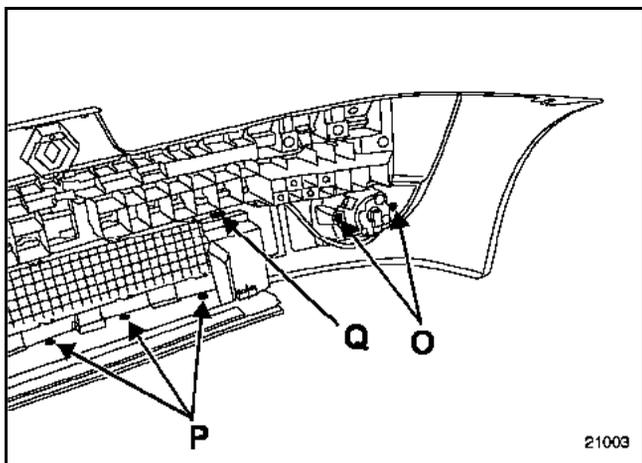
Remove the two mounting bolts (O), disconnect the connector, then remove the fog light.
