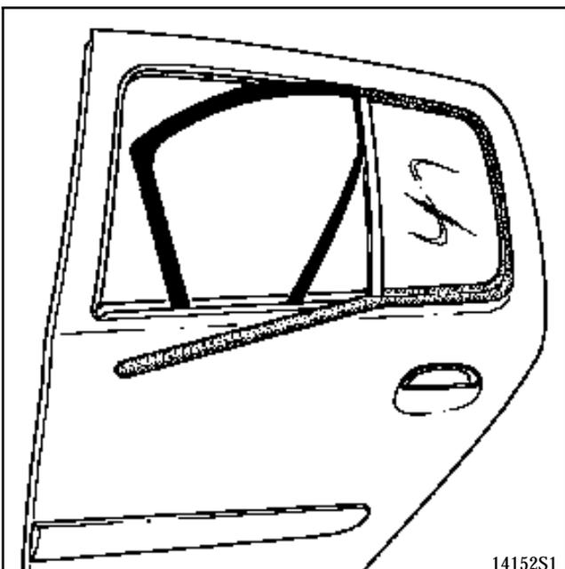
Remove the rear door window guide (see section 66-C).
