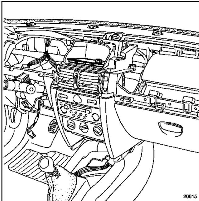
Unclip the Carminat keypad or the change tray (depending on the fittings) using grab handle removal tool (**Car.1597**).
