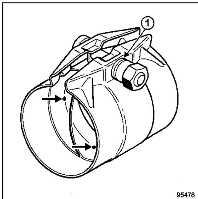
Place the sleeve end on the worn section of the pipe.
