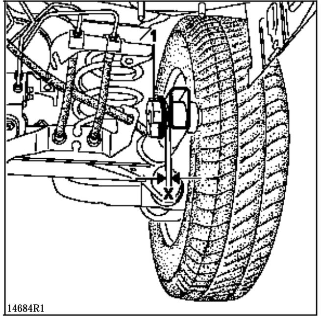
**IMPORTANT :** When refitting the rubber bush, avoid bringing the threaded rod section of the actuator screw to its end stop; it is preferable to unscrew the rod again and to move the actuator screw using the knurled section (this has the effect of making the pushrod section of the actuator screw go back in). Then re-screw again to completely refit the rubber bush.
