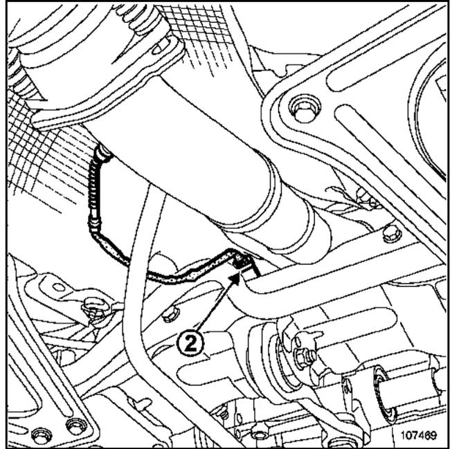
Disconnect the catalytic converter upstream oxygen sensor connector (2).
