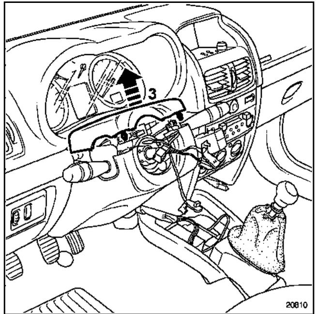
– the steering column upper half cowling, as shown above (3).
