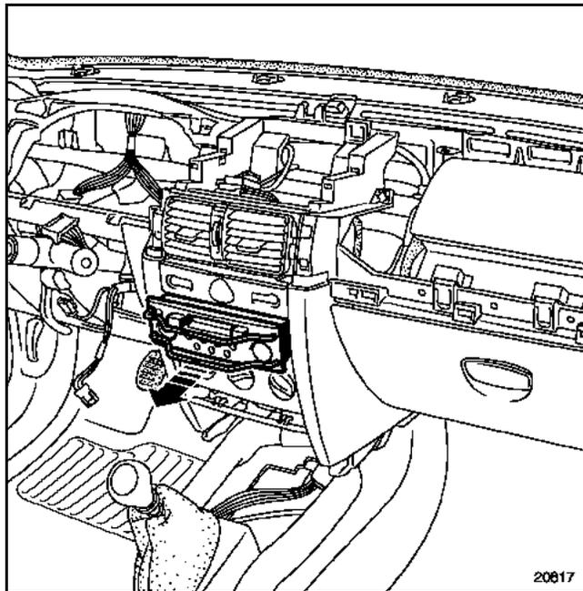
Remove the radio using tool (**MJ.1373**).
