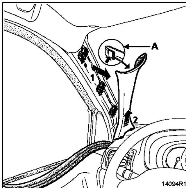
Partially remove the door seal.
