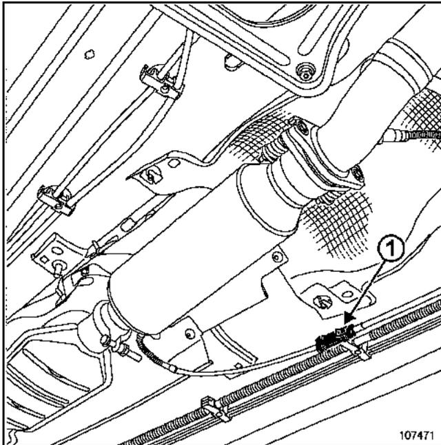
Disconnect the catalytic converter downstream oxygen sensor connector (1).
