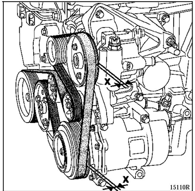
It is essential to turn the engine through two revolutions to position the belt correctly.
