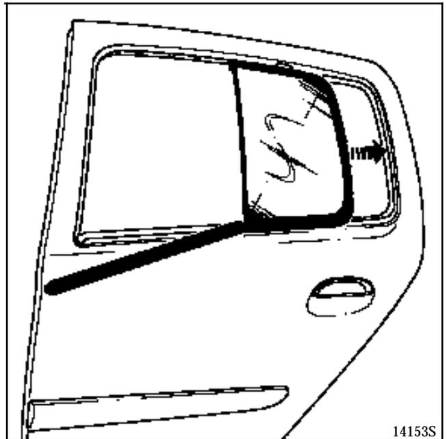
Before fitting the frame, ensure that the fixed window is correctly fitted.
