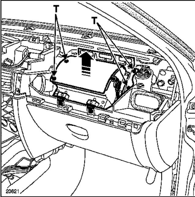
Position the mounting bolts (T) and tighten them to a torque of (6 N.m).
