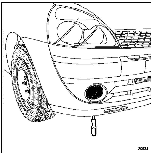
Adjust the two fog lights using a screwdriver.
