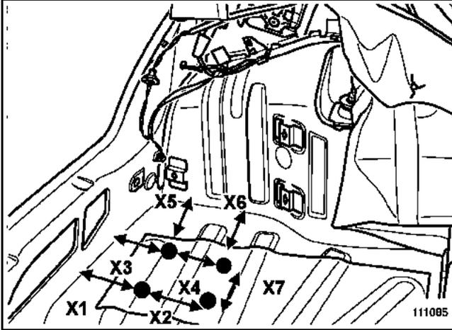
Place the floor flat on the boot floor and mark the location of the exhaust mountings on the boot floor, in accordance with the following measurements:
