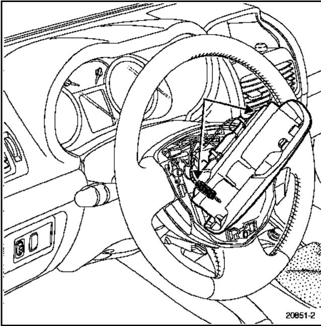
Disconnect the two generator power supply connectors.
